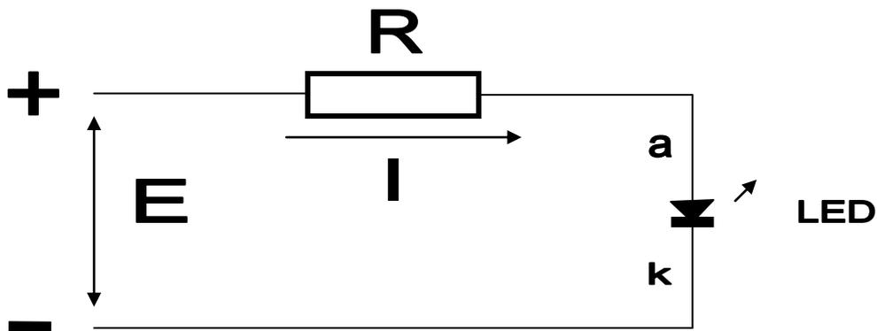
(Example only) - by Ohm's Law for a supply of 12 volts and allowing 2 volts drop across the LED for a forward current of 20 mA through the LED the required resistance would be 500 Ohms ( $12 - 2 = 10$ , divided by  $0.02 = 500$ ) The nearest common resistor is 470 Ohms or 560 Ohms.
